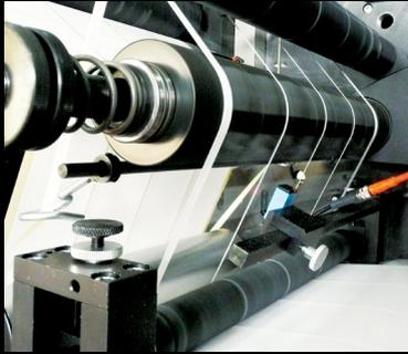
Shear - and razor blade cutting unit with easy setup feature
